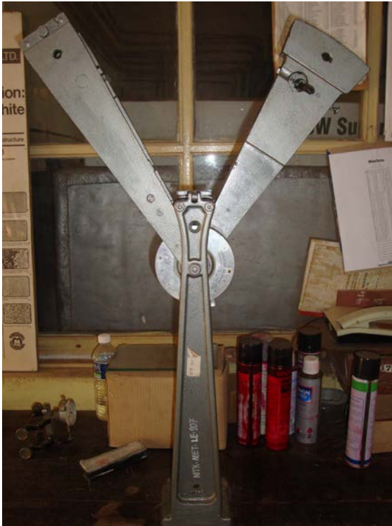
Figure 1: Hounsfield balanced impact testing apparatus used for measuring Impact strength.
